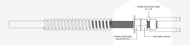
If the lip does not fully extend and does not engage the locking mechanism, loosen the spring compression locknut and turn the spring compression adjustment nut clockwise one-half turn. Check the operation of the ramp with this adjustment. Verify that the lip returns to its stored position without any problems when the ramp is lowered.
