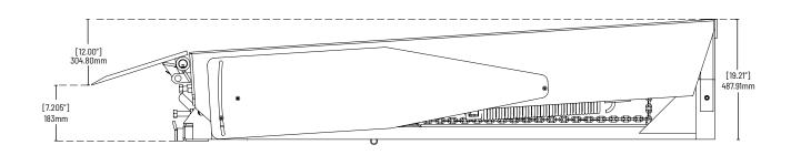
15.5" - 15.75" distance between lip end and bottom end of faceplate. Recommended distance for proper operation of the lip lock system and the tension settings established for the cane spring.
