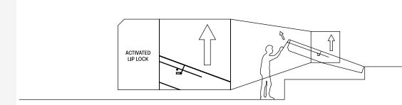
Once the lip is completely retracted, walk to the front of the ramp. The platform leveler will descend until the lip rests on the corresponding locks.
