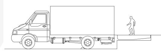
To bring the ramp below the platform level pull the release chain of the anti-fall mechanism on the middle front of the ramp and continue walking to the front of the ramp to lower it to the desired level.
