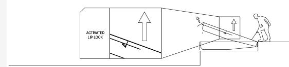
Once the leveler meets the height (12'), release the lip by lifting it manually, this will release the lip lock and then let it fall gently.
