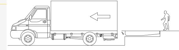
Once the lip is fully retracted and detached from the truck, pull the release chain gently to raise the leveler partially and walk to the front of the ramp. The platform leveler will descend until the lip rests on the corresponding locks.
