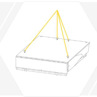
Using slings or chains for a minimum capacity of 1000 Kg, lift the ramp from the appropriate attachment points as shown below and carefully position it inside the pit. Make sure that the gap between the sides of the grader and the sides of the pit is equal. Also, check that the positioned shims are suitable for leveling the rear edges of the pit and leveler. Add or remove shims as needed.
