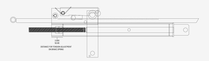
If the platform has too much movement when in any of the working positions or in the stowed position, the brake system may require adjustment. To make adjustments follow the process below. Using a 4" long die, for 1.125" nut
