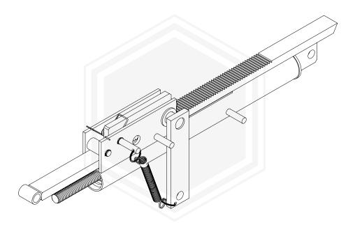
— The brake spring is set from manufacture at a distance of 2 inches as shown in the figure.
